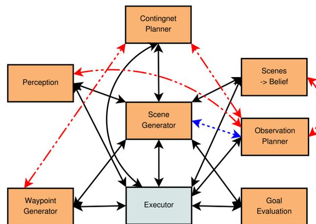
With one component fewer, the non-ontology version still has slightly more inter-component connections. Also the *complexity* of the interactions is much higher; components have a varying number of interactions with unpredictable other components.
